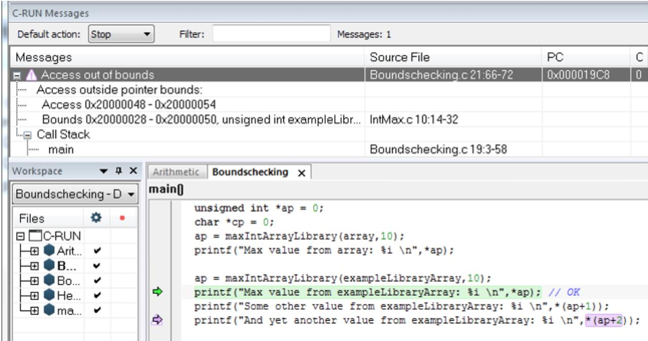
The screenshot displays the C-RUN Messages window and the source code editor. The Messages window shows an error: "Access out of bounds" in Boundschecking.c at lines 21:66-72. The source code editor shows the following code:
